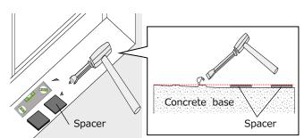
Remove any protrusions and level with spacers
