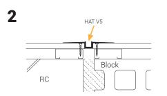
Mount the HAT V5 Joiner by inserting the protrusion into the gap between the boards.
