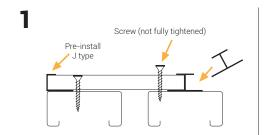
Pre-install J type on the edge of the board prior to starting H type installation. Then, loosely secure the board with screws (Don't fully tighten yet) and slide H type over onto the board so that the board sits firmly within the Joiner.
