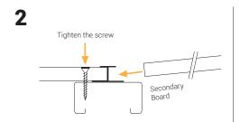
Tighten the screws and insert the second board into the Joiner.
