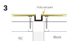
Apply putty and paint over the surface to cover the wings of the HAT V5 Joiner.
