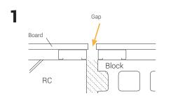
Install the boards leaving the appropriate gap for the HAT V5 Joiner.
