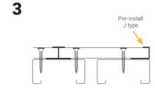
Pre-install the  ${\bf J}$  type on the edge of the last board. Secure the second board with screws.
