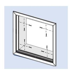
**5**Create the lid (insert the board into the inner frame and attach it With the board retainers)
