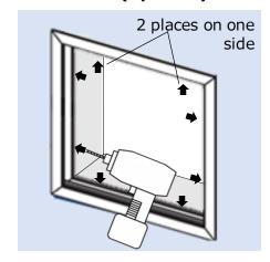
**4**Secure with screws on the inside the frame
