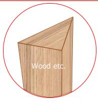
Concrete tends to leak between the formwork and the chamfer before it hardens
