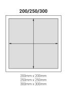
Note: All 3 sizes (200, 250, 300) are available in 2 different configurations, 1 for use with 9.5mm board and 1 for use with 12.5mm board.
