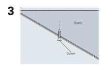
Secure the ceiling board (e.g., gypsum board) to the ceiling.
