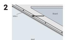
Insert ceiling board (e.g., gypsum board) into the secured MIKIRI.
