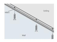
Secure **MIKIRI** to the ceiling along the wall with screws.
