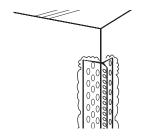
Attach to corner of concrete foundation.
